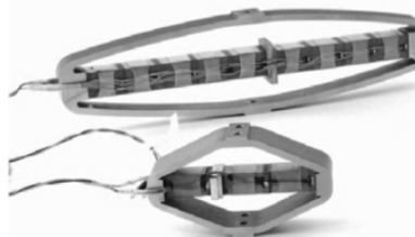
Figure 4.58. Piezoelectric linear actuators with amplitude amplification
