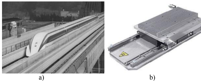
Figure 4.1. a) Maglev vehicle with linear motor propulsion – MLX Japan; b) linear motor for machine-tools
