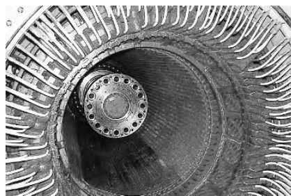
Figure 7.11. Motor-generator with water supply by tubes in the stator bars
